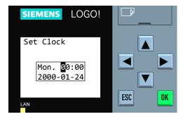
Step 5: To select the value to be changed, press ◀ or ▶. To change a value, press ▲ or ▼. When finished, press the "OK" key.
