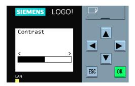
**Step 5:** To adjust the contrast, press **◄** or **▶**. When finished, press the "OK" key.
