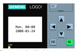
**Step 1:** Press **▼** repeatedly until the display does not change. To begin the configuration process, press the "**ESC**" key.
