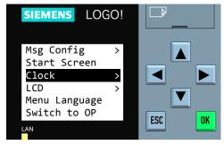
Warning: Do not select "Switch to OP". Doing so will remove the ability to set the clock. If this is selected by accident, the password to set the mode back to ADMIN is "LOGO".
