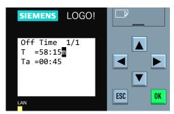
**Step 6:** The cursor will blink in the set value. To select the digit to be changed, press ◀ or ▶. To change the value of a digit, press ▲ or ▼.
