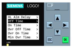
Step 4: Press o r to select the desired parameter to adjust and press "OK". Continue to Step 5 on the following pages for the specific block type being edited.
