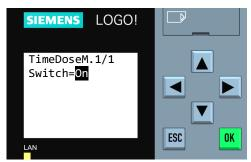
Step 5: The bottom line indicates the current state of the softkey switch. In this example, the softkey is set to "On". To change the set value for the parameter, press the "OK" key.
