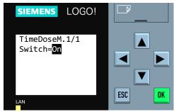
Step 6: The cursor will blink on the switch parameter. To change the set value has been changed from "On" to "Off".
