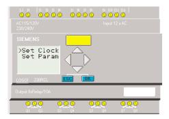
Step 2: Two options will be given. The arrow on the LCD display will point to "Set Clock." Press the "OK" key.
