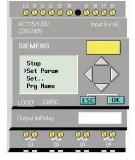
Step 2: Press ▼ on the unit to select "Set Param." Then press the "OK" key.
