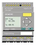
Step 3: Press ▲ or ▼ to view the parameter values. In this example, "Off Time" is being viewed.
