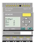
Step 4: The first line indicates the on threshold for the parameter. In this example, the "MinOCycl" is 3, "On = 3." To change the set value for the parameter, press the "OK" key.
