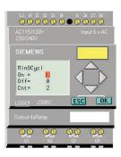
Step 5: The cursor will appear in the set value. To select the digit to be changed, press ◀ or ▶ . To change the value of a digit, press ▲ or ▼ . In this example, the set value has been changed from 3 to 2.
