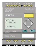
Step 6: When the desired time value has been entered, press the "**OK**" key. The new time value will now be in effect.
