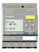
Step 4: The first line indicates the set value for the parameter. In this example, the set time is 1 hour and 55 minutes, "**T=01:55h**." To change the set value for the parameter, press the "**OK**" key.
