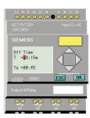
Step 5: The cursor will appear in the set value. To select the digit to be changed, press ◀ or ▶ . To change the value of a digit, press ▲ or ▼ . In this example, the set value has been changed from 1 hour and 55 minutes to 58 minutes and 15 seconds. (The timebase can be changed from hours = h to minutes = m or seconds = s by moving the cursor to the far right and pressing ▲ or ▼).
