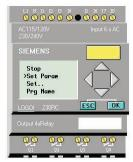
Step 2: Press ▼ on the unit to select "Set Param." Then press the "OK" key.
