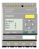
Step 6: When the desired counter value has been entered, press the "**OK**" key. The new value will now be in effect.
