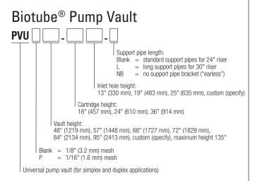
Orenco's Biotube Pump Vault is available in standard and customized configurations. Contact Orenco or your nearest distributor for sizing recommendations.
