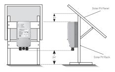
Figure 3: Pentair Pentek Solar Drive Mounting
