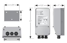
Figure 4: Pentair Pentek Solar Drive Dimensions
