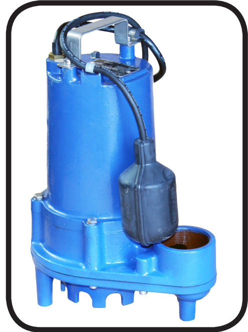
Submersible Effluent 2" Discharge, 3/4" Spherical Solids Wide Angle Float
