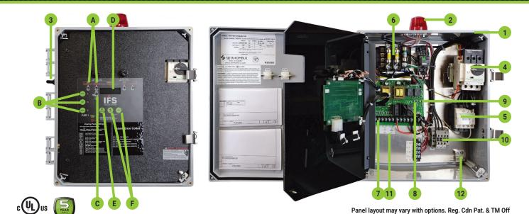
The IFS simplex control panel utilizes an innovative circuit board design to control one 208/240/480 VAC three phase pump in water and sewage applications. IFS panels feature an easy-to-use touch pad on inner door for programming and system monitoring. The panel configuration can be easily converted in the field to either a timed dose or demand dose. Available with the EZconnex® float system.
