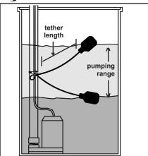
Due to weight of cable, pumping range <u>above</u> horizontal is NOT equal to pumping range <u>below</u> horizontal. Use values published on front page as a guide. Pumping ranges are based on testing in non-turbulent conditions. Range may vary due to water temperature and cord shape. Note: As the tether length increases, so does the variance of the pumping range.
