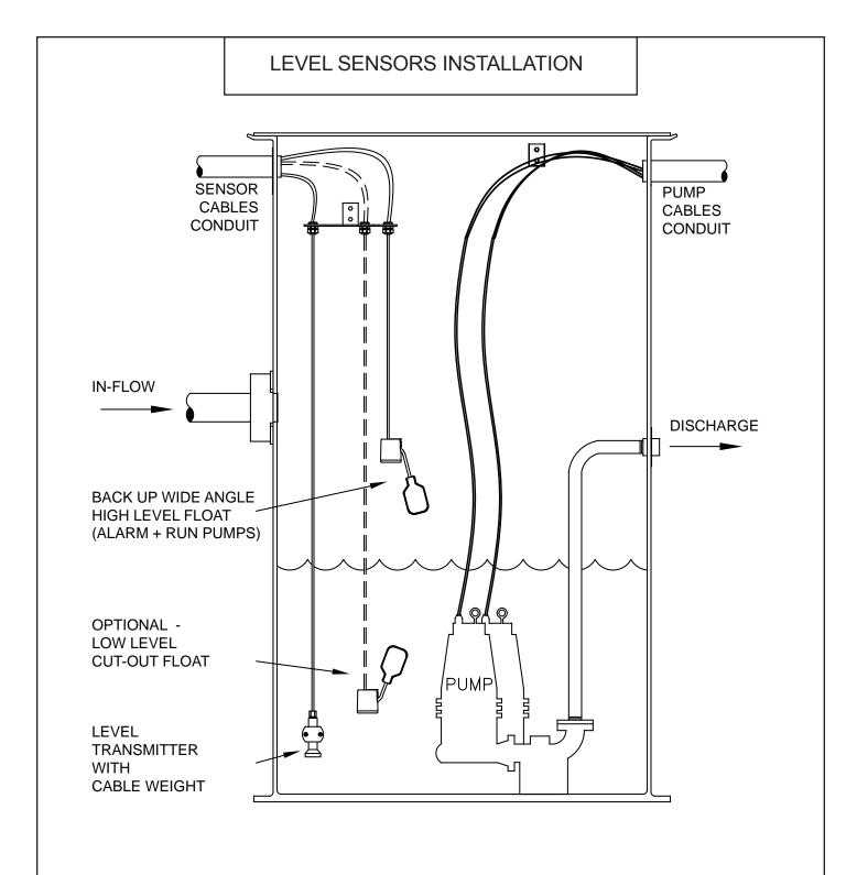
Typical transmitter (with high level float back up) setup for a duplex lift station
