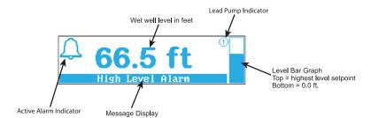
The main screen displays the set well level and any active alarms. The controller will return to the main screen automatically after 3 minutes of inactivity.
