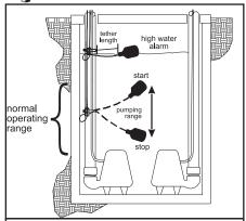
Due to weight of cable, pumping range <u>above</u> horizontal is NOT equal to pumping range <u>below</u> horizontal. Use values published as a guide. Pumping ranges are based on testing in nonturbulent conditions. Range may vary due to water temperature and cord shape. Note: As the tether length increases, so does the variance of the pumping range.
