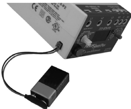
Figure 4: Proper Position of the Battery Cable
